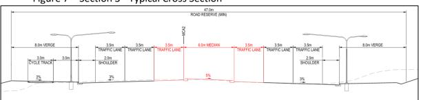
Figure 7 – Section 3 - Typical Cross Section
