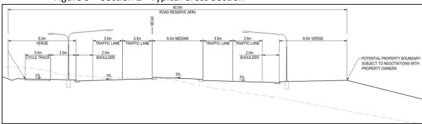
Figure 5 – Section 2 - Typical Cross Section
