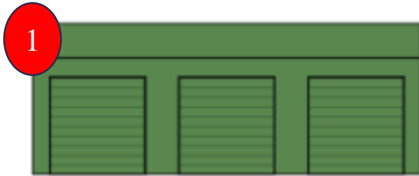
ELEVATION 1 – NORTHERN – 12m wide – 3 door opening, 6m wide awning over (not to scale)
